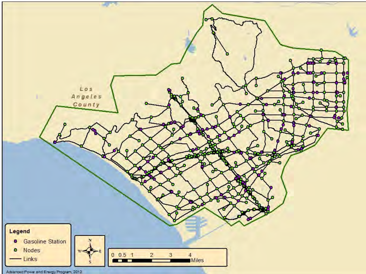
Figure 40: Coarse Roadway Network of Road Segments and Intersections Used to Determine Optimum Hydrogen Station Locations in the Santa Monica Region
