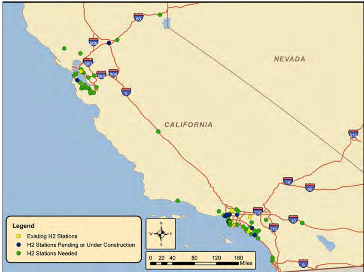
Figure 1: Location of 18 Existing and 50 Additional Hydrogen Fueling Stations Required in California by 2015 to Enable Commercial Volumes of Fuel Cell Electric Vehicles Shown for the Entire State
